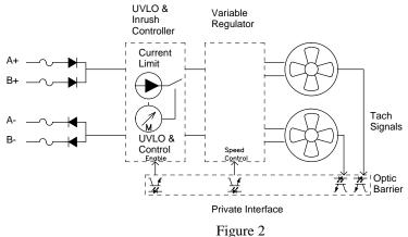
It is the control section that is different. While a much less complex control and interface section is required, the system must have specialized hardware to interface to the fan tray. Some data would need to be reported as not available or gathered outside the tray. A temperature sensor would be an example of how this could be done. Another approach would be to use a single private I2C bus, as shown in Figure 3, which could give nearly all the features of the IPMB
